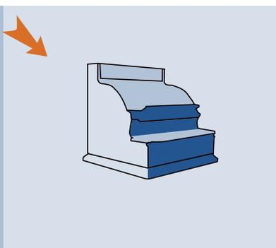
If the distribution of the Baltic spotlight is changed to a 12 degree beam the light intensity is higher. More detail is revealed but is also less subtle. The shadow becomes sharper.
