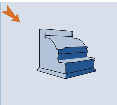
The ambient lighting is created by the same wall scalloping and spill light. More detail is revealed with the addition of a 24 degree beam Baltic spotlight lighting from the left. More texture is revealed, also sparkle. It also adds a shadow to the display.
