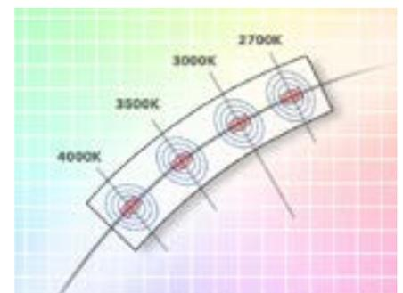
Corrected Cold Phosphor Technology® Xicato XSM modules perform to less than a 2 step MacAdam Ellipse as illustrated.
